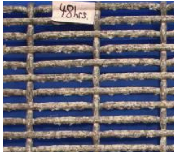
J&L Standard Floor Panel After 48 hours (Enlarged to Show Deterioration of Coating)
