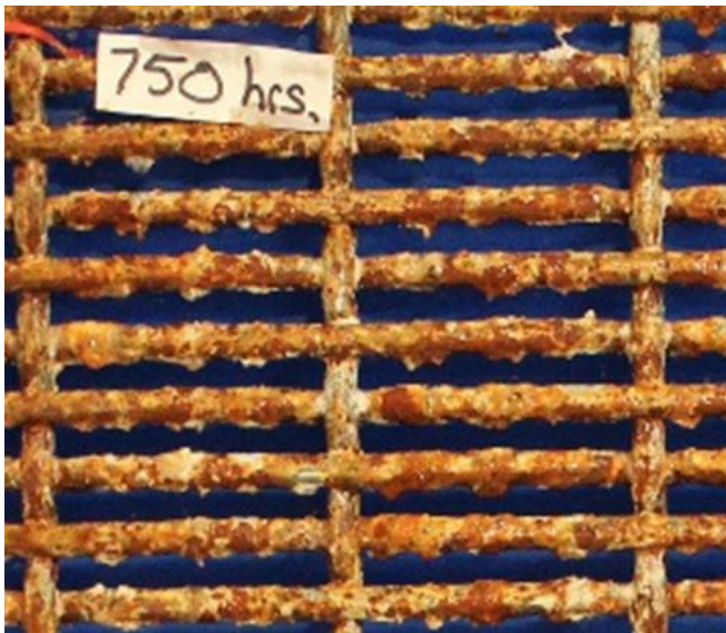
J&L STANDARD FLOOR 750 Hours Exposure Extensive Corrosion (red rust)
