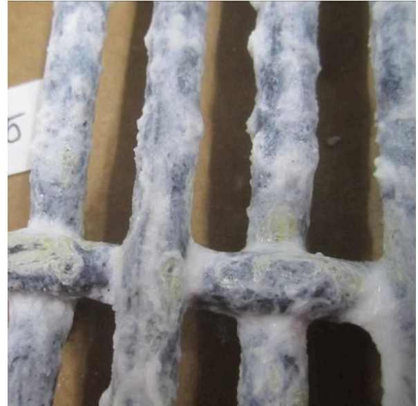
J&L BOSS HOG EXTRA™ Improved Floor Panel After 552 hours (Enlarged to show protective coating)
