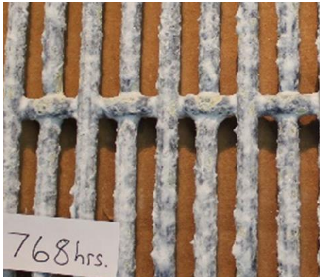
J&L IMPROVED FLOOR PANEL (BOSS HOG EXTRA™) 768 Hours Exposure Signs of Yellowing Powdery Oxide Seen from Protective Coating
