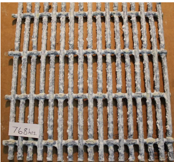
J&L BOSS HOG EXTRA™ Improved Floor Panel After 768 hours
