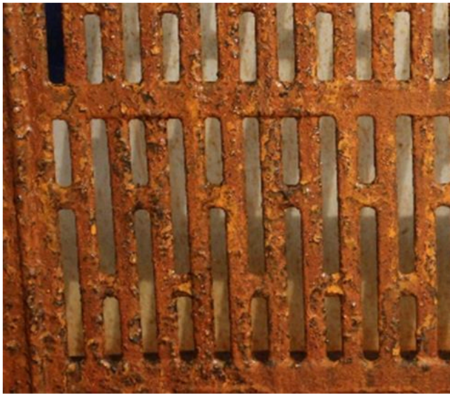
COMPETITOR #1 750 Hours Exposure Extreme Corrosion of Base Metal
