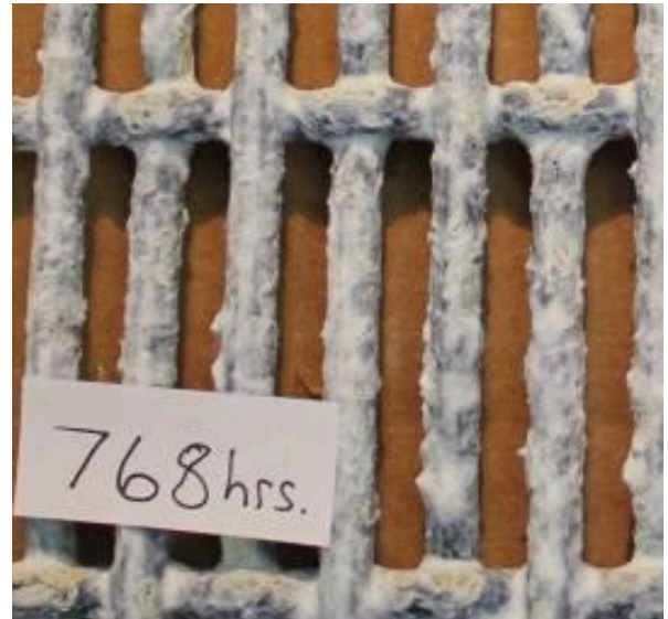
J&L BOSS HOG EXTRA™ Improved Floor Panel After 768 hours (Enlarged to show protective coating)
