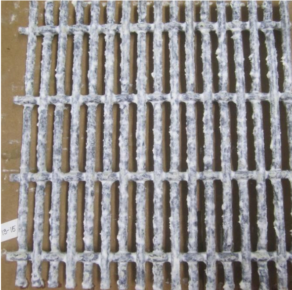
J&L BOSS HOG EXTRA™ Improved Floor Panel After 552 hours
