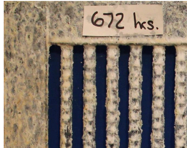
COMPETITOR #2 Triangular Floor Panel After 672 hours (Enlarged to show formation of red rust)
