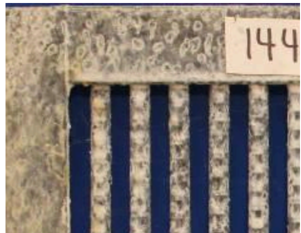
COMPETITOR #2 Triangular Floor Panel After 144 hours (Enlarged to show beginning yellowing)
