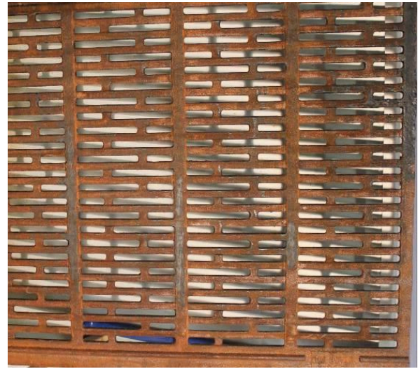
COMPETITOR #1 Cast Iron Floor Panel After 48 hours
