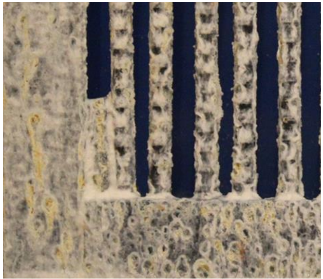
COMPETITOR #2 750 Hours Exposure Some Corrosion (red rust) Powdery Oxide Seen from Protective Coating
