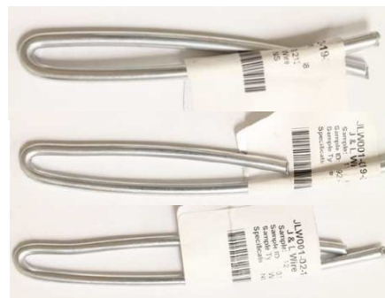
ZINC-COATED No Peeling Observed PASSED Bend Test
