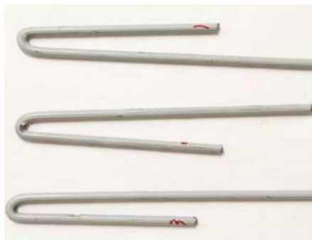
PAINTED Peeling Observed at Bend FAILED Bend Test
