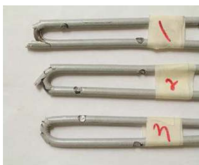
POWDER-COATED Peeling Observed at Bend FAILED Bend Test
