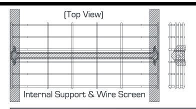
The wire screen fits tightly to the inside wall of the rack beam. It is formed to install under the top of the beam leaving a level surface that is even with the top of the beam.
