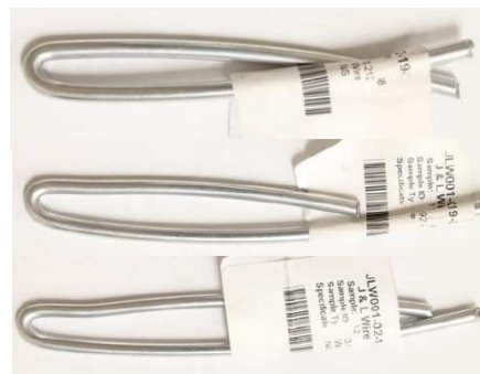
ZINC-COATED No Peeling Observed PASSED Bend Test
